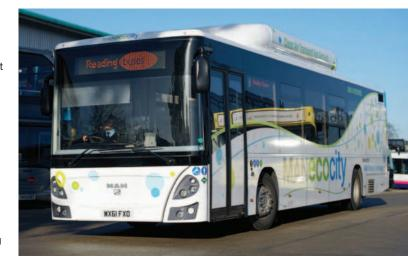
MAN's EcoCity was designed and constructed specifically for the UK market. MAN claims operating cost savings of some 30% and the ability to run on the UK's fast-building supplies of biogas – thus reducing emissions to zero.
